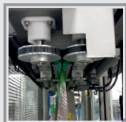
bag separation unit with V-belt
